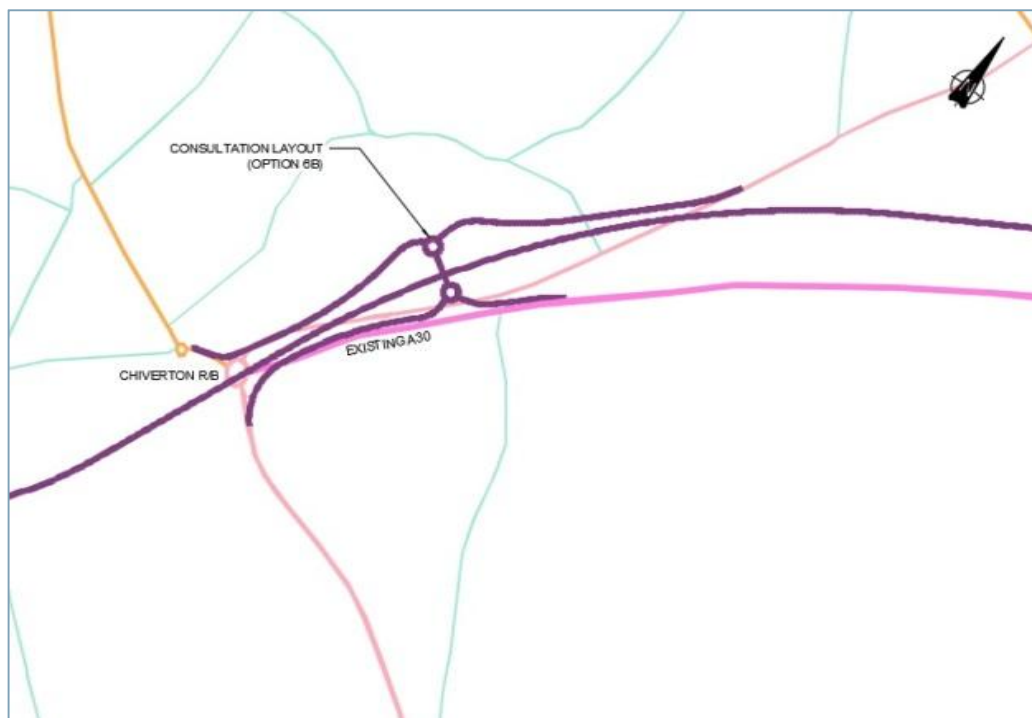
Figure 7-2: Chiverton junction - alternative large gyratory layout
