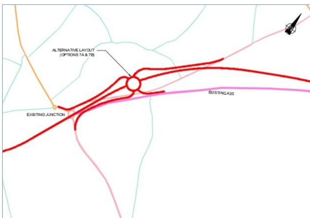
Figure 7-2: Chiverton junction - alternative large gyratory layout
